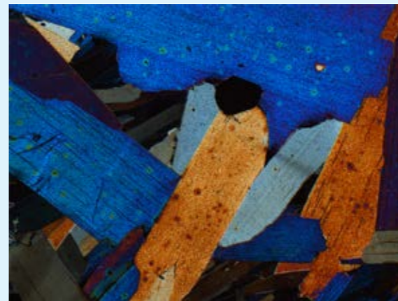
Figure 20: Interlocking mica textures in a potassium-altered 1.53 billion year old intrusion, northern Queensland, Australia. Dark circular patches are caused by radiation damage around inclusions of zircon. Cross polarised light image
