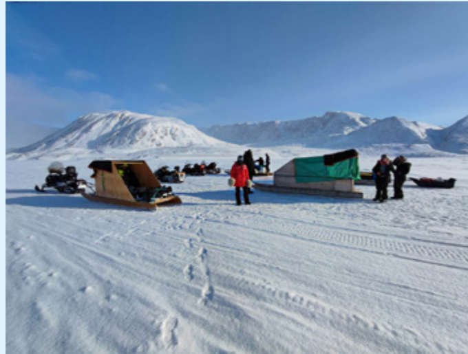
These sleds are used in some locations when travelling on the frozen sea around Baffin Island. These are towed by snowmobiles and are able to carry people and equipment and provide some protection from the strong winds
